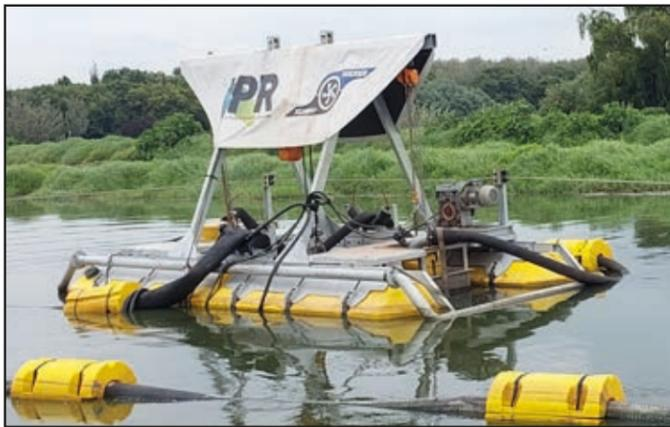
the SlurrySucker MK III boasts enhanced solids handling capabilities. The pumps are fitted with robust cutter fans or agitators, facilitating the management of larger particles. Moreover, they can effectively handle slurries with a high specific gravity (SG).
